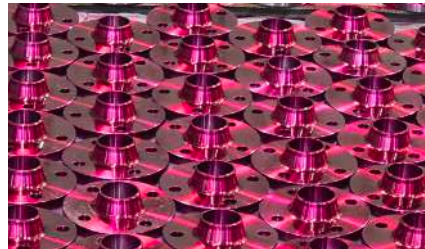
Liquid penetrant Test
